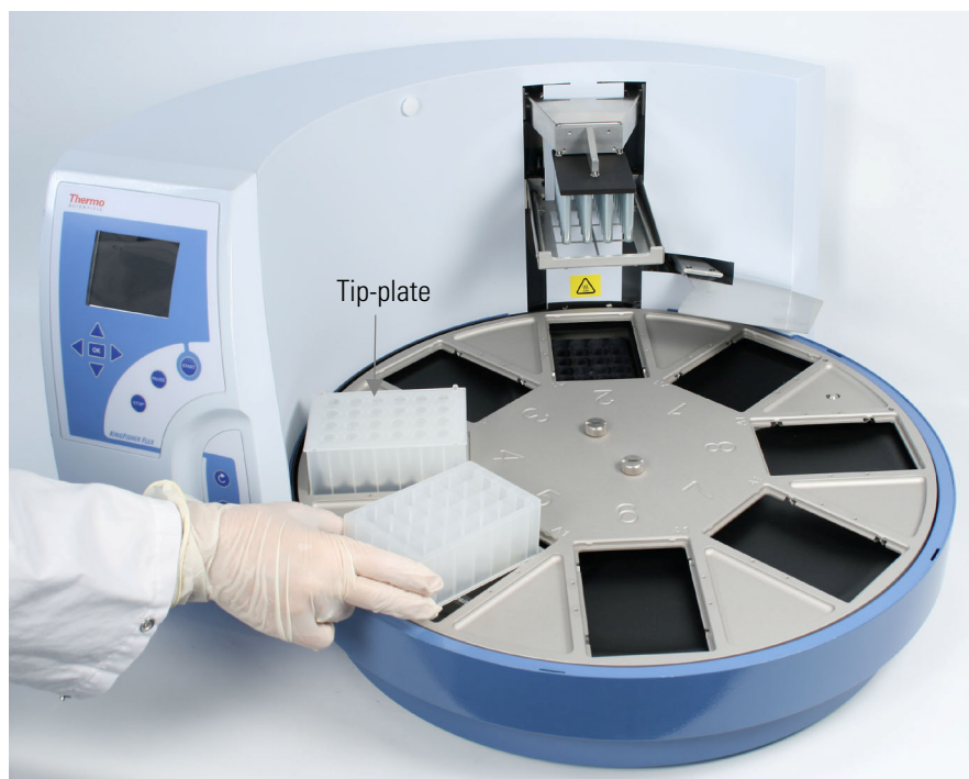
Figure 4-41. Loading the plates
