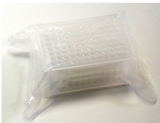
Figure 4–33. Tip comb package with two tip combs
