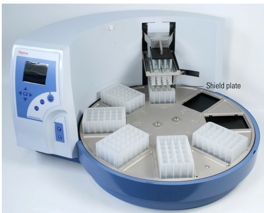
Figure 4-44. Shield plate in function
