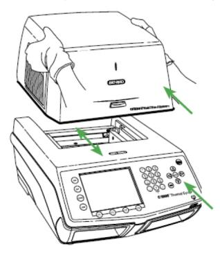
Pull up the locking bar until it is flush with the sides of the module bay. This action moves the module forward, locking it into place.
