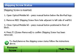
2. Follow the instructions to remove the shipping screw. The following diagram shows the location of the shipping screw.
